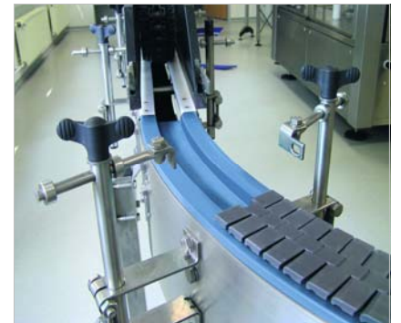
LubX® C: Curve guide for POM conveyor chain
