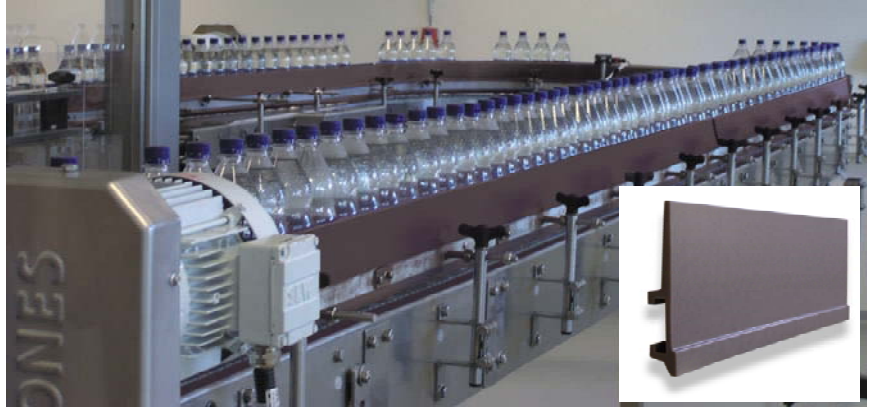
Bottling plant: LubX® S rail guide aligned of the sliding partner PET
