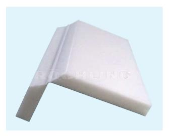
**Integrated hinge:** Foamlite® P has an "integrated" hinge. It is sufficient to mill a simple 90-degree V-notch into it. The high bending fatigue strength of the material means that the hinge can be folded more than 40,000 times without breaking.
